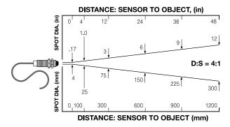
D:S is the optical resolution expressed as a ratio of the distance to the resolution
