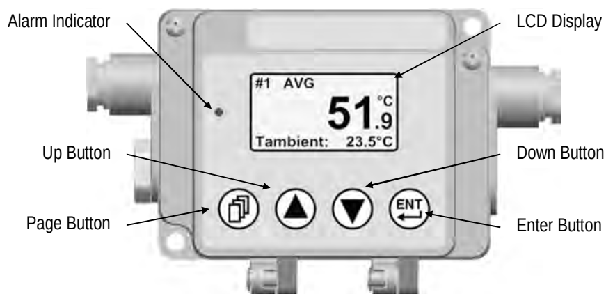
Figure 32: Control Panel for the Comm Box (metal)
