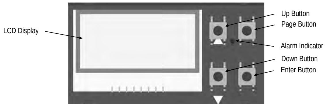
Figure 33: Control Panel for the Comm Box (DIN)
